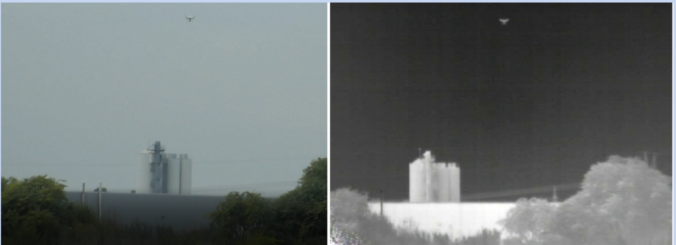
Figure 1: This example shows the same objects in two different spectral ranges: VIS (left) and LWIR (right). Even if some details are better highlighted in VIS spectral range (because the imager has a higher resolution), the visual contrast between different objects is better in LWIR (thermal contrast between drone and sky, building and sky or foliage and wall are better than their reflective contrasts).
